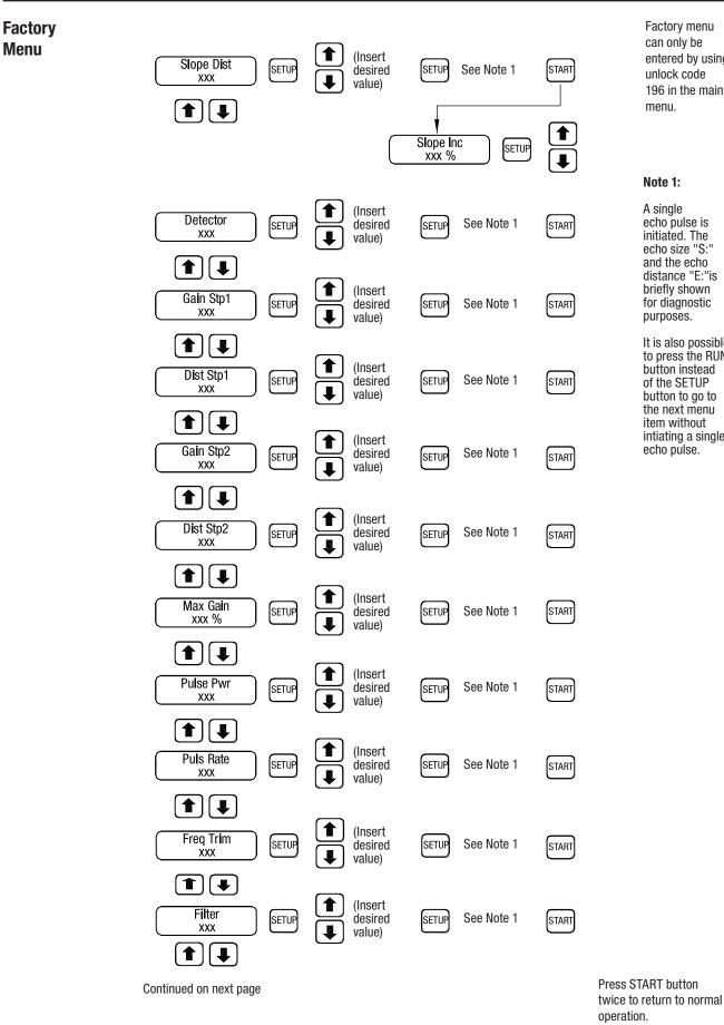
Factory menu can only be entered by using unlock code 196 in the main menu.
